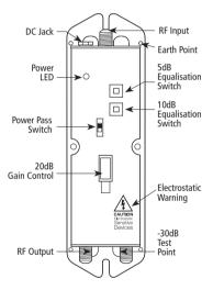
The DA43 is an economical, low noise GaAs wide-band distribution amplifier for use in digital television systems. It features a 20dB gain control and up to -15dB of cable equalization. (see Fig. 1).
